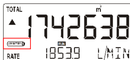
Fig. 4: Low-battery alarm (typical)
