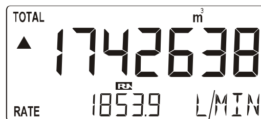
Fig. 3: Process information (typical)
